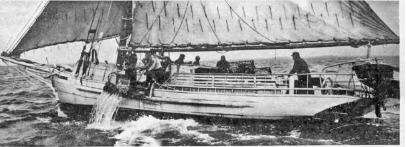
The Leonard was built in Dorchester county in 1882. She is 45 feet long. Captain Jones has owned her for 35 years, using her for oyster dredging. Here the dredge is being brought up after a run across Stone Rocks, off Sharps Island in the bay.
